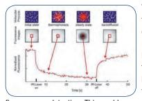
The technology uses a fluorescence microscope equipped with a dichroic mirror that couples a IR-Laser into the path of fluorescence light. The heating laser is focused with the same objective used for
